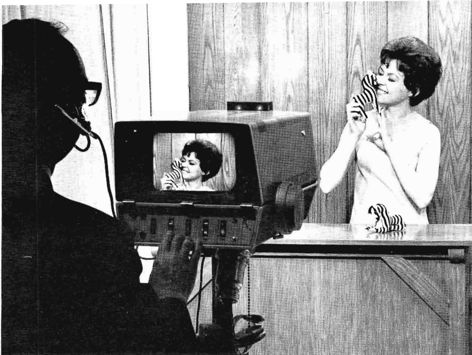
FIG. 1 Lightweight and compact, the PK-330 Studio Camera produces crisp, high-resolution pictures. The camera has built-in pan and tilt functions and a motorized zoom lens.
