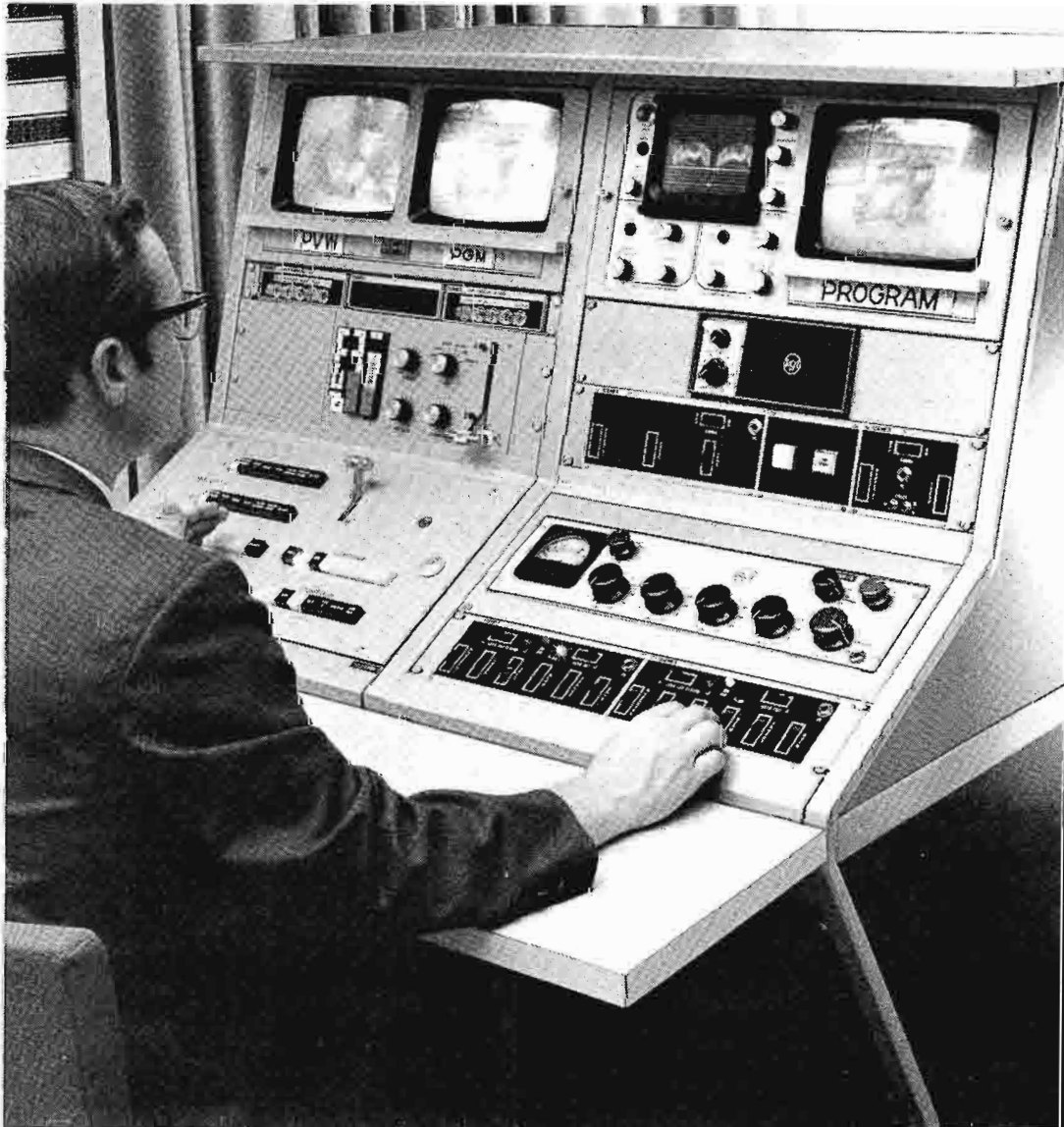
FIG. 8 PTC Series Consoles are functional and attractive. A removable front shelf permits rolling the consoles through a standard 36 inch door.
