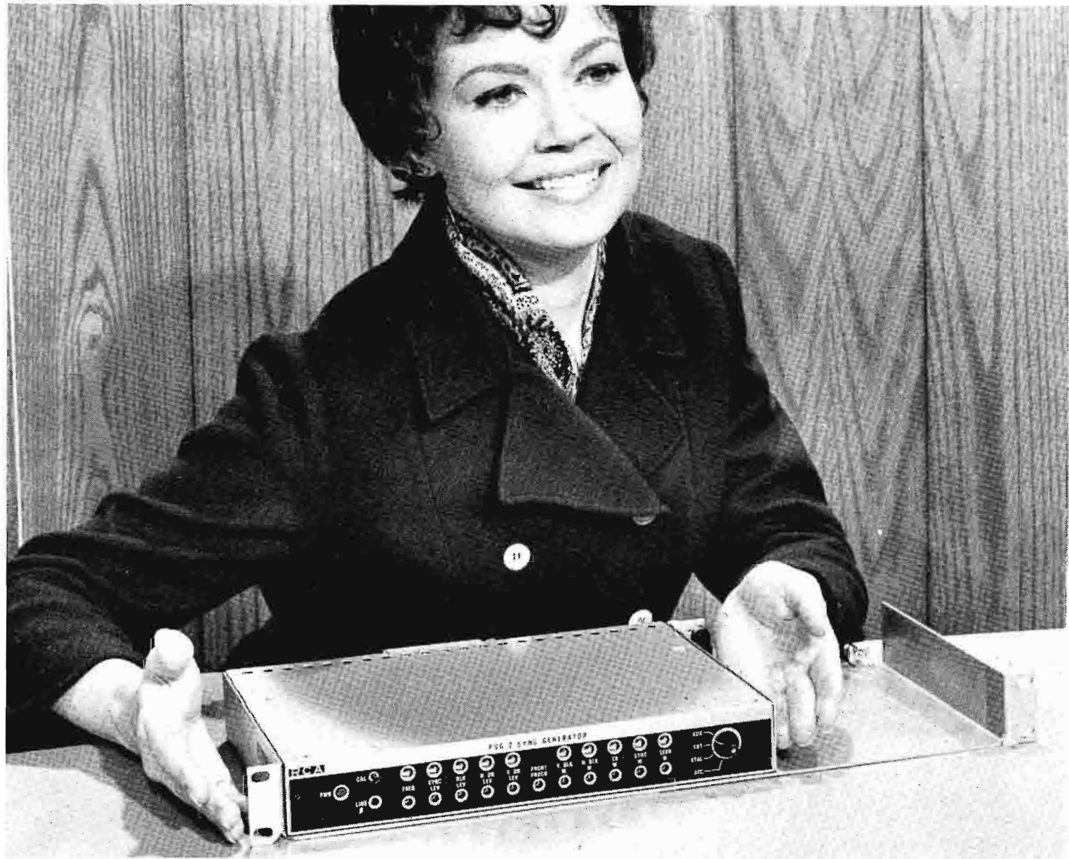
FIG. 7 Newest member of Professional Television's terminal equipment line is the PSG-2 Sync Generator. It occupies only \frac{2}{3} of a rack-mounting space 1\frac{3}{4} inches high and produces all four pulses needed for operation of monochrome television installations.
