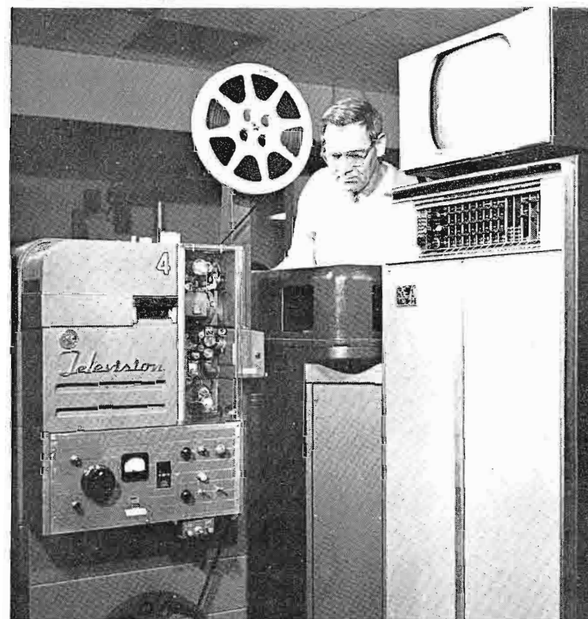
FIG. 5 KOB-TV Color Film/Slide chain using TK-27 Color Camera, TP-15 Multiplexer, TP-7 Slide Projector, and TP-6 16mm Film Projector.
