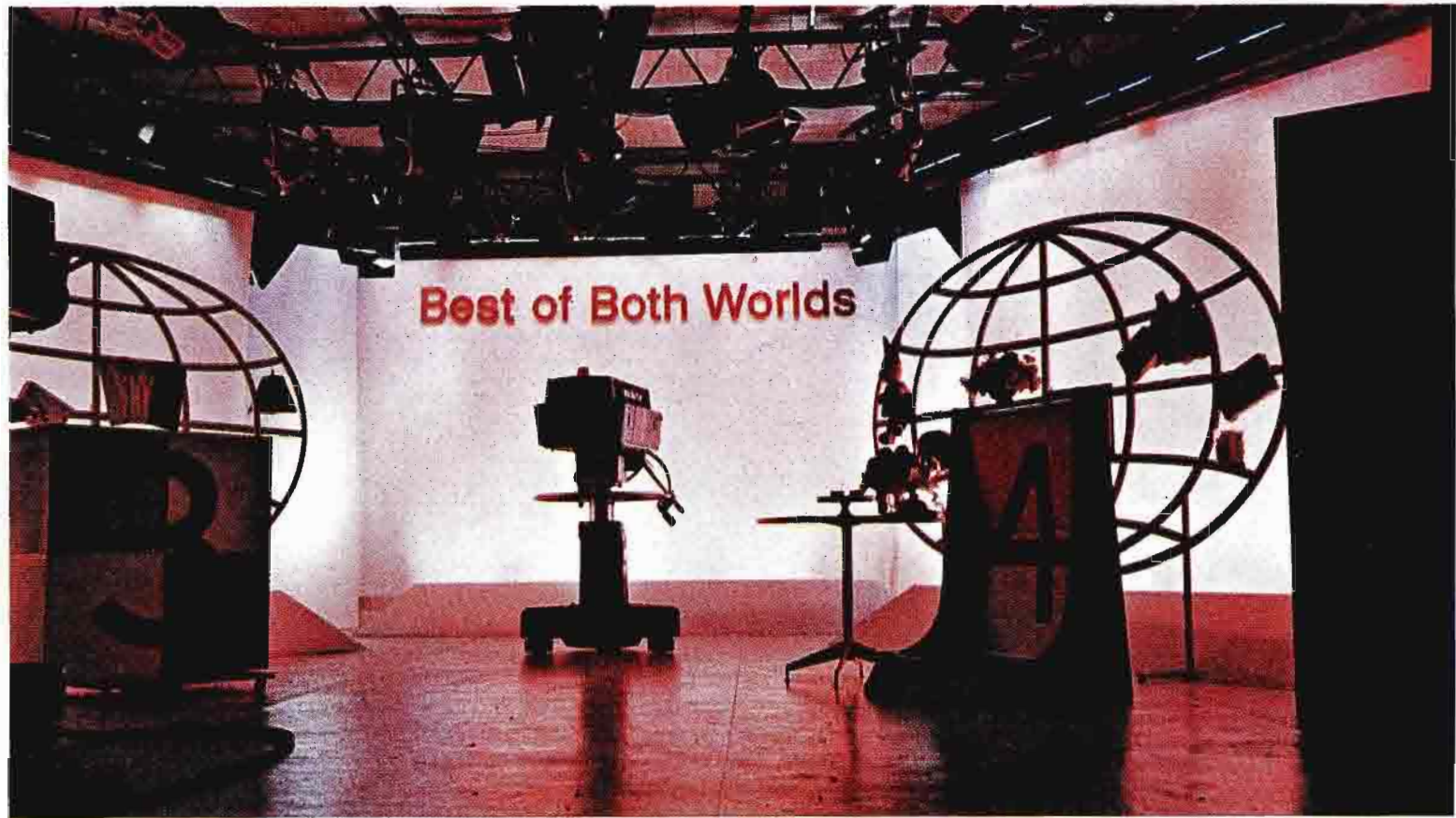
CYC AND SCRIM enclosed the color demonstration studio. Striplights, overhead and floor, used new plastic gels, in the primary colors, to produce a wide variety of color backgrounds. Quartz fixtures, supplied by Colortran, were used throughout the studio. The basic simplicity of the set demonstrated the kind of sophistication color lighting can bring to color TV pictures.
