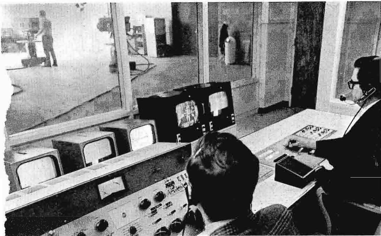
FIG. 16 Each studio has its own control room as shown above, containing the BC-8 audio console, PTS-1 switching system, remote controls for VTRs and film chains.
