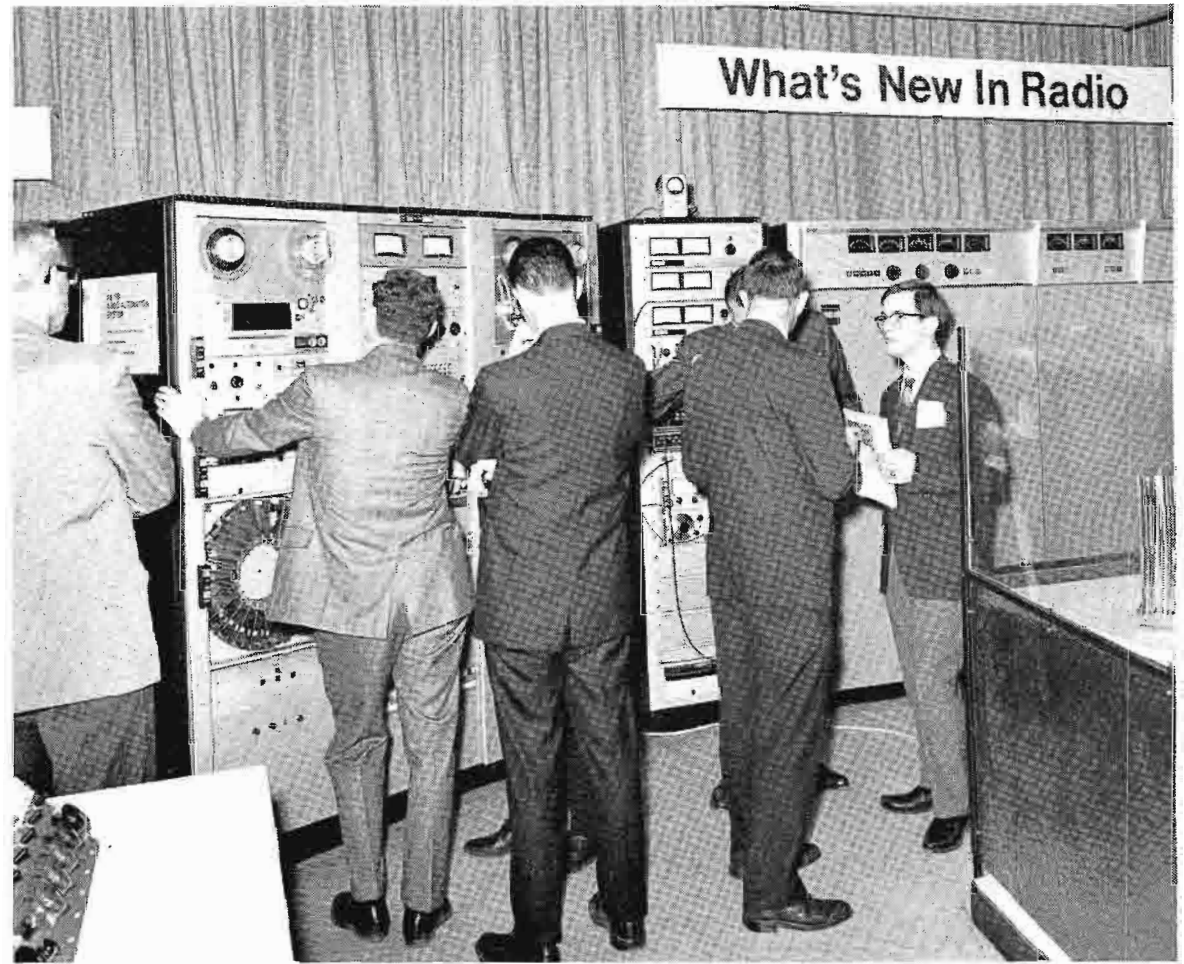
NEW SOLID-STATE RADIO EQUIPMENT that carried out the "What's New in Radio" theme were the new RCA AM/FM Audio Automation System using solid-state logic and relay switching, a new solid-state FM Exciter, Stereo Generator, SCA Generator and new wideband solid-state FM Monitors. The broadcasters showed a tremendous amount of interest in this area throughout the show.
